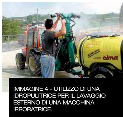
IMMAGINE 4 – UTILIZZO DI UNA IDROPULTRICE PER IL LAVAGGIO ESTERNO DI UNA MACCHINA IRRORATRICE.
